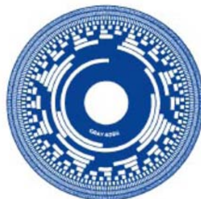
Figure 5: Code disc for an optical absolute encoder features one track for each bit of resolution. The number of bits n ( 2n ) corresponds to 2n radial positions.
